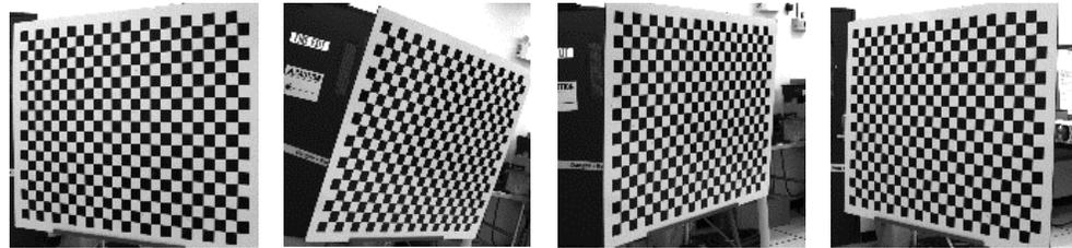
2. Algorithm solves for best fit focal length and fits residual error to a distortion model
