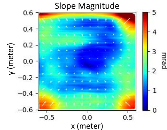
Example SOFAST measurement of entire heliostat
